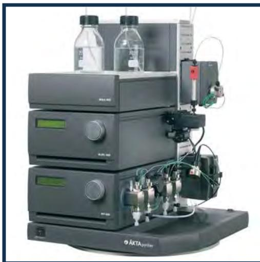
**Figura 24.** Sistema Akta Purifier 10-UPC de GE Healthcare®
