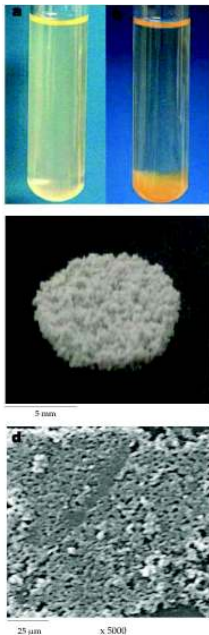
Figure 6. Sulfated polysaccharide from Navicula sp. before (a) and after (b) the addition of \text{FeCl}_3 ; lyophilized gel (c); SEM micrograph of the lyophilized gel (magnification \times 5000 , scale bar 25\ \mu\text{m} ) (d).
