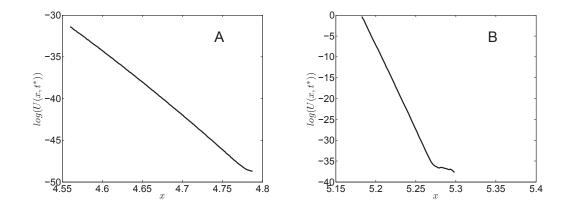
Figure 4.2: Exponential behavior of the solution of equations (3.1) and (4.1) at the location of the fronts. (a) Karma model. Domain  $x \in [0, 120]$ . Slope  $m_K = -84$  approximately; (b) MV model. Domain  $x \in [0, 200]$ . Slope  $m_{MV} = -417$  approximately.
