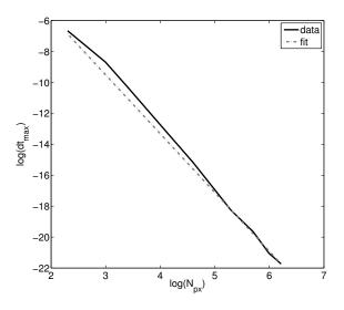
Figure 5.7: Behavior of  $dt_{max}$  as a function of  $N_{px}$  in a log-log scale along with the respective fit  $dt_{max} = c (N_{px})^a$ . For this case,  $c \approx 1.8838$  and  $a \approx -3.8$ .
