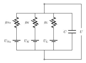
Figure 1.1: Electrical circuit to model the membrane of an excitable cell;  $g_{Na}, g_K$ and  $g_L$  are the conductances for sodium, potasium and leakage current, respectively, and,  $U_{Na}, U_K$  and  $U_L$  represent the Nernst potential for each respective ion. U and C are the potential and the capacitance of the membrane, respectively.
