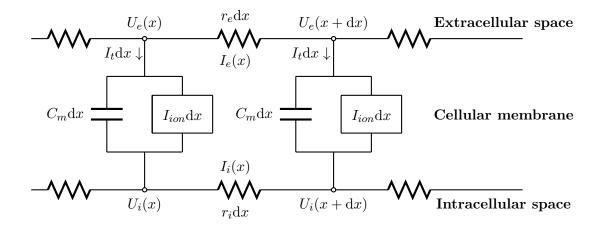
Figure 1.2: Circuit that models the cable equation
