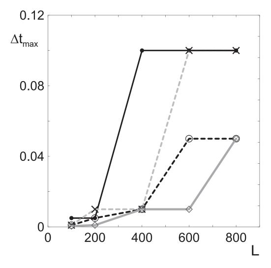
Figure 4.4: Maximum  $\Delta t$  in order to obtain a stable solution for the Karma model using the CMD method for different values of length of the domain *L*, fixed  $N_{cx} = 4$ ,  $N_{ix} = 299$  (Solid black),  $N_{ix} = 499$  (dashed gray),  $N_{ix} = 699$  (dashed black),  $N_{ix} = 899$  (Solid gray).
