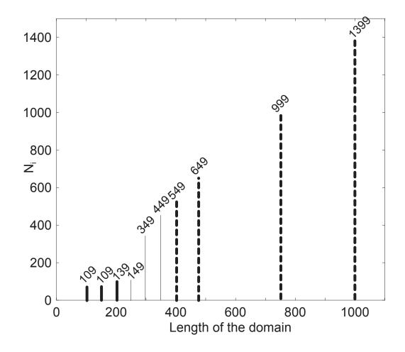
Figure 4.3: Number of subintervals  $N_i$  (with  $N_c = 4$ ) in order to get precision of  $O(10^{-2})$  as a function of the length of the domain, for the Karma model (Eq. 3.1). Solid Bold ( $\Delta t = 1 \times 10(-2)$ ), Solid ( $\Delta t = 1 \times 10(-3)$ ), Dashed Bold ( $\Delta t = 1 \times 10(-4)$ )
