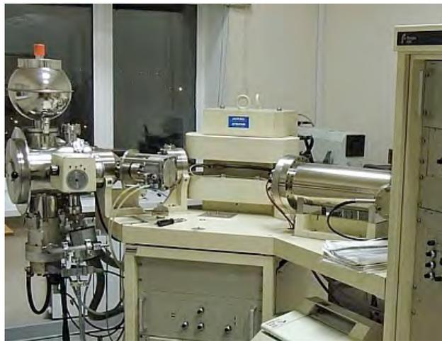
**Figura 1.5:** Finnigan MAT 262 Thermal Ionization Mass Spectrometry (TIMS).
